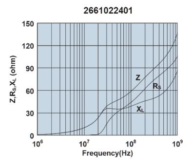
Impedance, reactance, and resistance vs. frequency.
