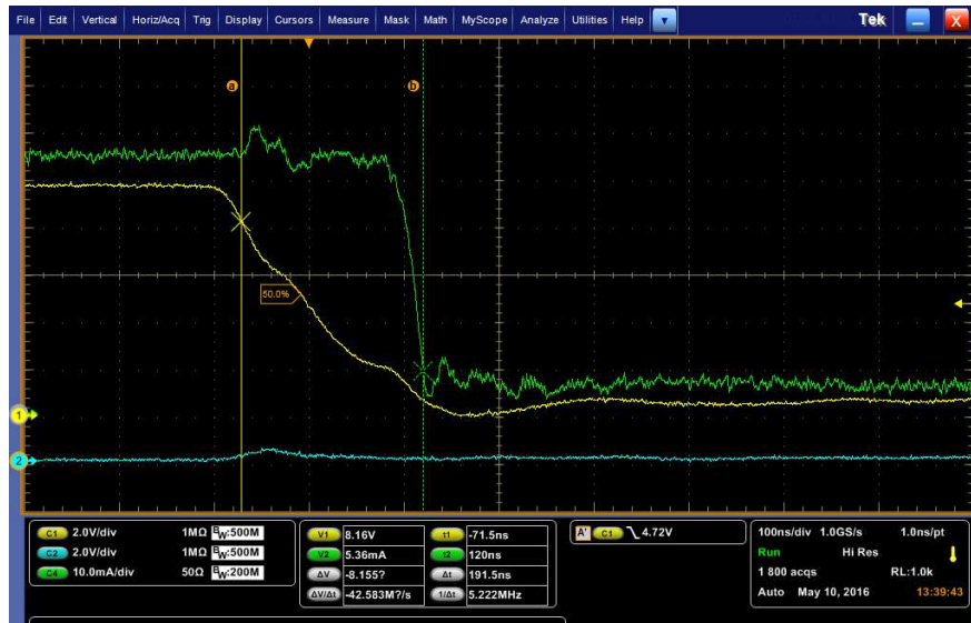
Figure 7. Turn Off Time of BCR401/2/5 While Switching the Power Path as Shown in Figure 3c
