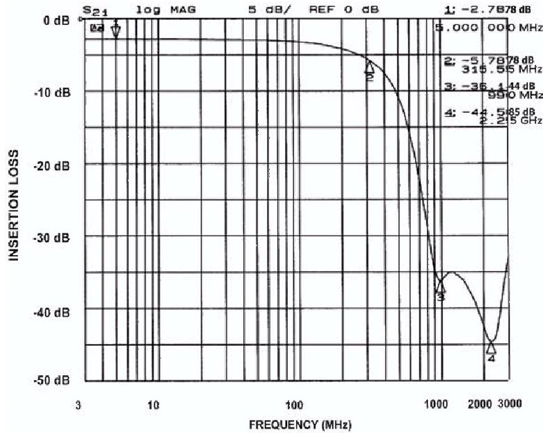
Figure 2. Insertion Loss vs. Frequency (Pins 2 and 15)
