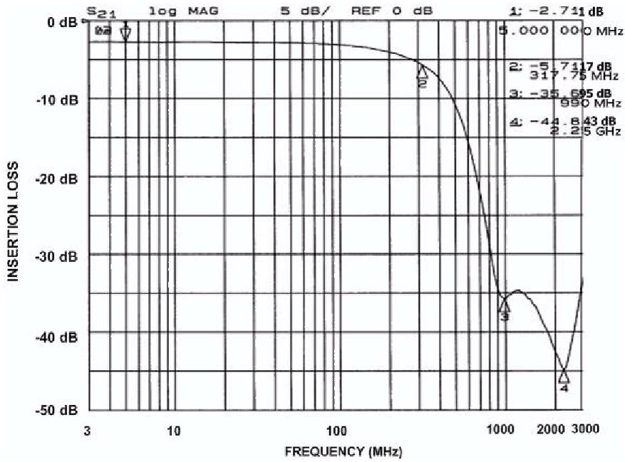
Figure 4. Insertion Loss vs. Frequency (Pins 6 and 11)
