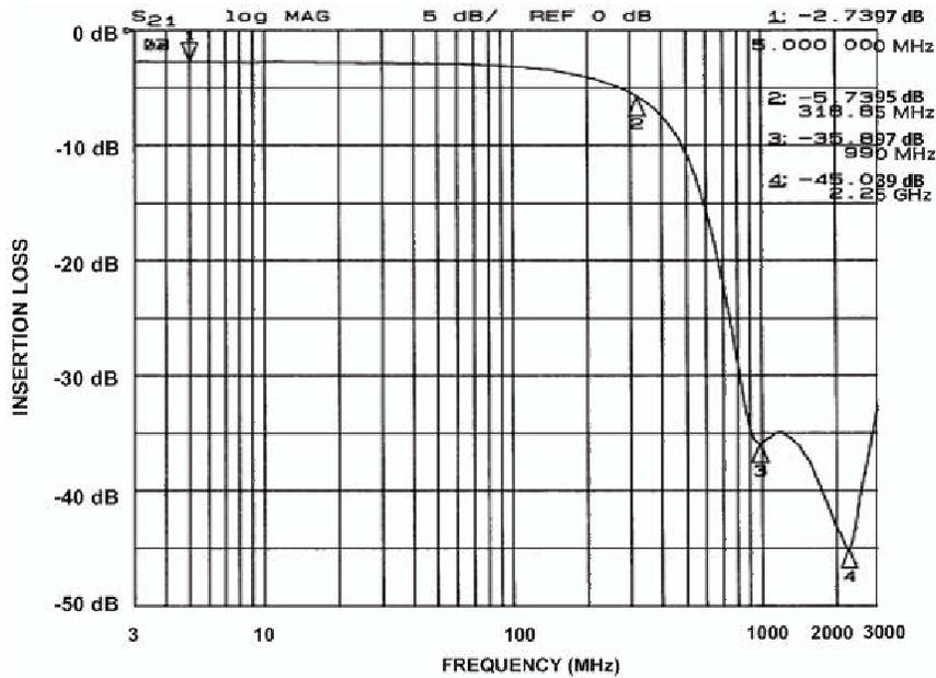
Figure 6. Insertion Loss vs. Frequency (Pins 8 and 9)
