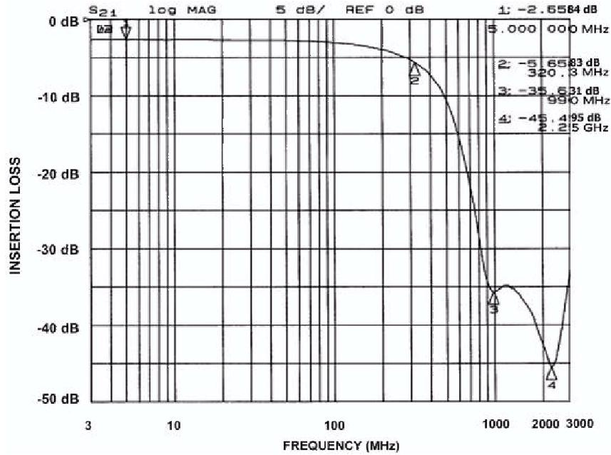
Figure 3. Insertion Loss vs. Frequency (Pins 3 and 14)
