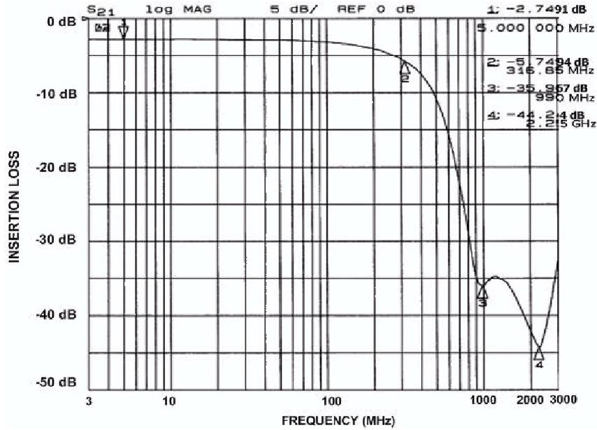
Figure 5. Insertion Loss vs. Frequency (Pins 7 and 10)
