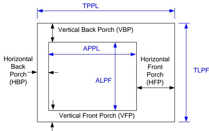
**Figure 1. Timing Parameter Diagram**
