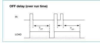
This function allows delayed switch-off of the relay. The configured value indicates the time elapsing between activation and switch-off. Information: An overrun is desired in many applications, e.g. to give some orientation with illuminations even after switch-off or to give a load enough time to complete the switch-off process.
