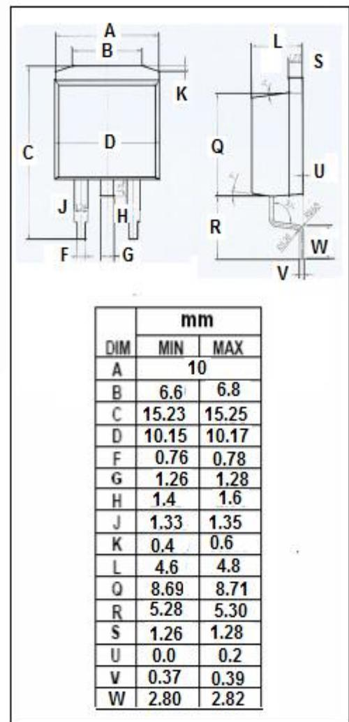
**isc N-Channel MOSFET Transistor**
