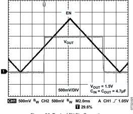
Figure 28. Typical EN Pin Operation
