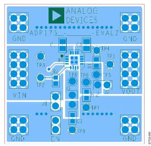
Figure 47. Typical Board Layout—Top Side
