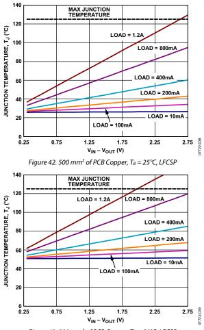
Figure 43. 500 mm<sup>2</sup> of PCB Copper,  $T_B = 50^{\circ}$ C, LFCSP
