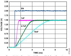
Figure 26.  $V_{\text{OUT}}$  Ramp-Up with External Soft Start Capacitor
