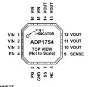
0 NOTES 1. NC = NO CONNECT. 2. THE EXPOSED PAD ON THE BOTTOM OF THE LFCSP ENHANCES THERMAL PERFORMANCE AND IS ELECTRICALLY CONNECTED TO GND INSIDE THE PACKAGE. IT IS RECOMMENDED THAT THE EXPOSED PAD BE CONNECTED TO THE GROUND PLANE ON THE BOARD. 07722-003
