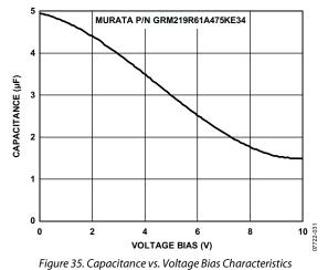
Equation 3 can be used to determine the worst-case capacitance, accounting for capacitor variation over temperature, component tolerance, and voltage.
