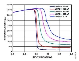
Figure 14. Ground Current vs. Input Voltage (in Dropout), Vout = 2.5 V
