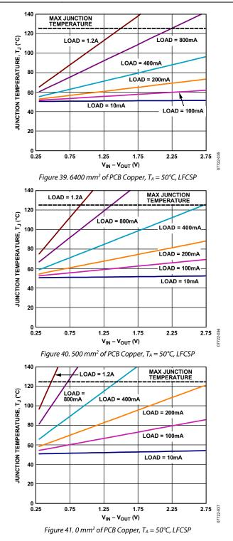
In cases where the board temperature is known, the thermal characterization parameter,  $\Psi_{JB}$ , can be used to estimate the junction temperature rise. Maximum junction temperature  $(T_J)$  is calculated from the board temperature  $(T_B)$  and power dissipation (P<sub>D</sub>) using the following formula:
