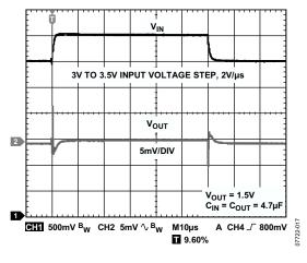
Figure 17. Line Transient Response, Load Current = 1200 mA
