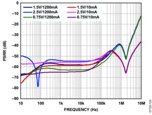
Figure 23. Power Supply Rejection Ratio vs. Frequency and Output Voltage
