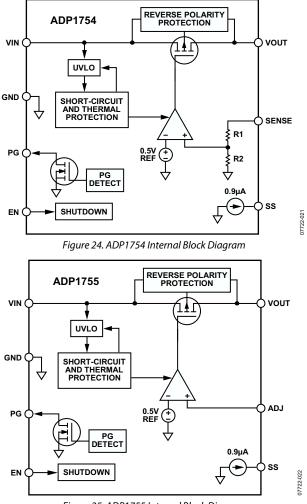
Figure 25. ADP1755 Internal Block Diagram
