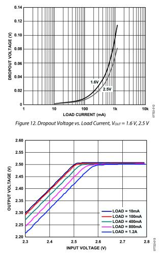
Figure 13. Output Voltage vs. Input Voltage (in Dropout),  $V_{OUT} = 2.5 V$
