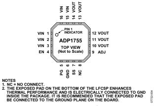
Figure 4. ADP1755 Pin Configuration
