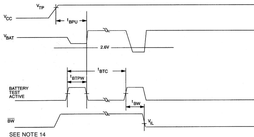
**POWER-DOWN/POWER-UP TIMING**(T<sub>A</sub>: See Note 10)
