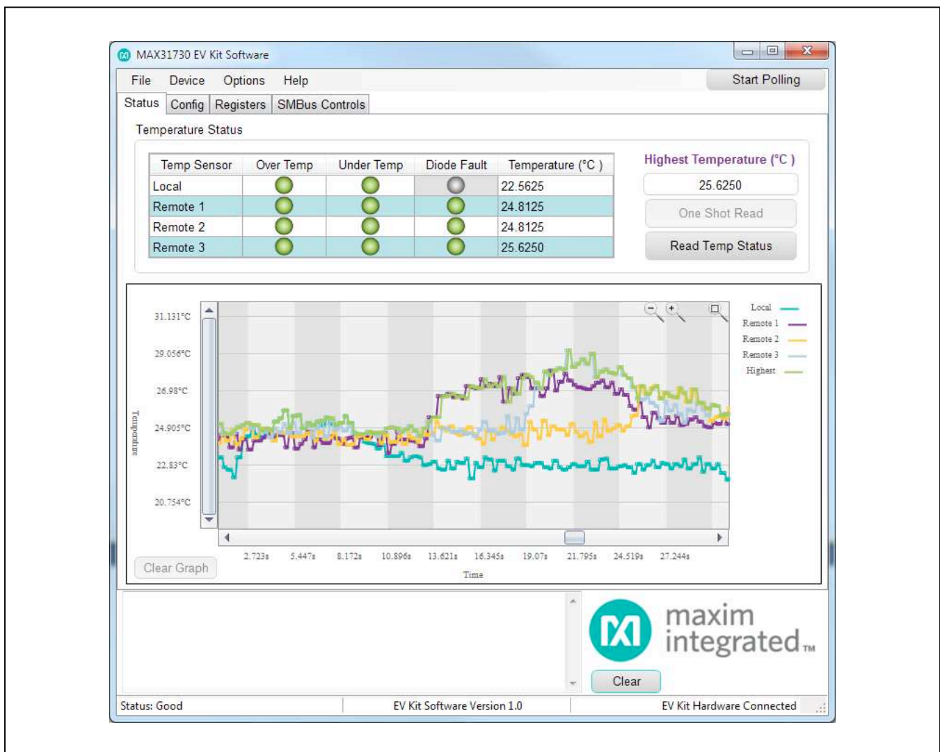
Figure 1. MAX31730 EV Kit Software GUI (Status Tab)
