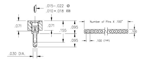
**Description:** Interconnect Socket Low Profile Solder Tail Socket Accepts .015" - .022" (0,38 - 0,559 mm) dia leads Single Row Through Hole Plating Code: Shell Plating: 10 μ" Gold over 100 μ" Nickel
