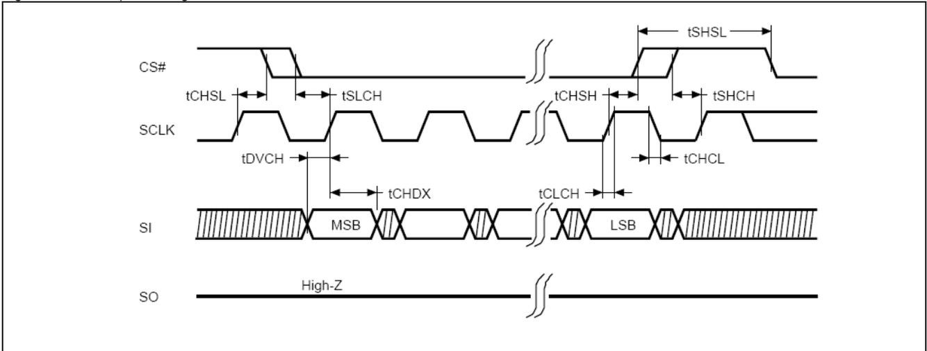
Figure 8. Output Timing
