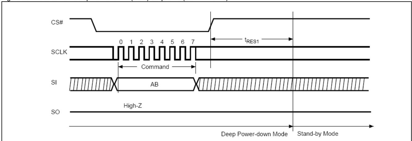
Figure 24. Release from Deep Power-down and Read Electronic Signature (RES) Sequence (Command AB)
