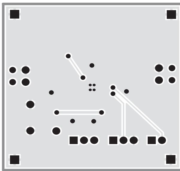
Figure 7: AAT2556 Evaluation Board Bottom Side Layout.
