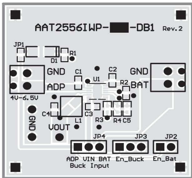
Figure 6: AAT2556 Evaluation Board Top Side Layout.
