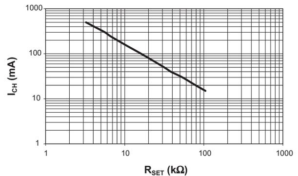
**Figure 2: Constant Charging Current vs. Set Resistor Values.**
