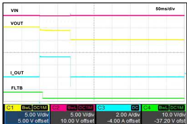
Figure 12. Over Current Protection (Latch-off)
