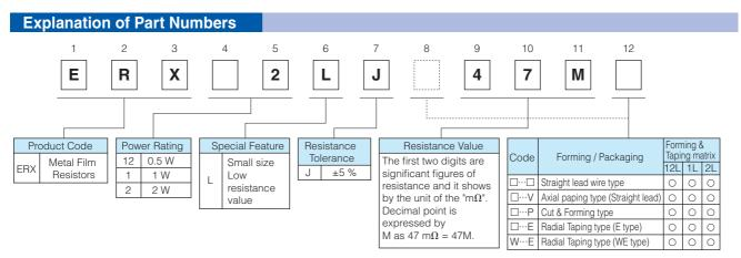
The above example shows a small size and low resistance value metal film resistor, 2 W power rating, resistance value of 47 m ohms, tolerance ±5 %, and package of standard bulk packing.
